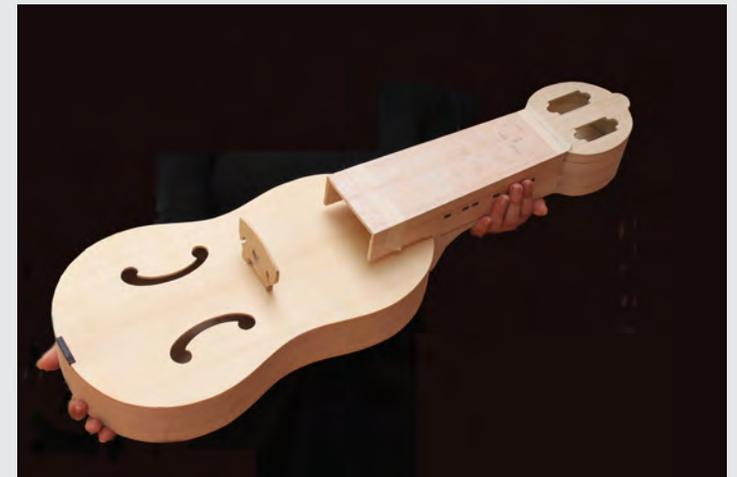
The keyboard, constructed in maple was conceived as an autonomous element, and to facilitate the varnishing it was varnished separately, and assembled when this was completed.
