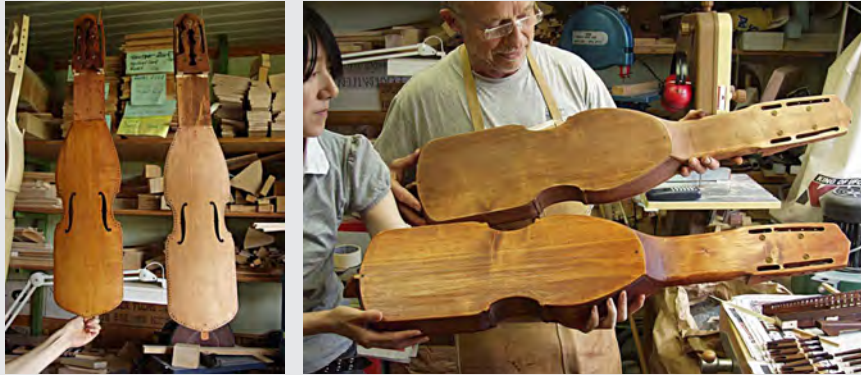
Before and after applying shellac on top of the stain color. Shellac change the color to more yellow and red.
