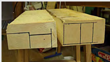
Above: The sides can be cut out from a thick spruce plank
