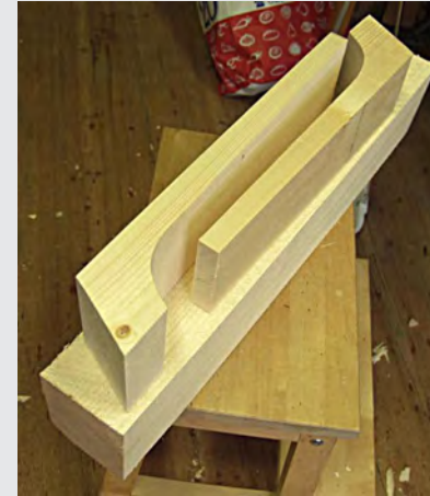
Left: 2 necks are cut out with a band saw
