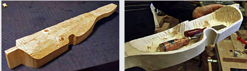
To make a copy of an old nyckelharpa, "Gammelharpa", you have to work directly on the full spruce log. It takes an awful lot of hard work to hollow out the inside.
