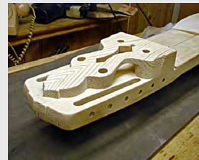
Below: Reinforcement for the tuning pegs
