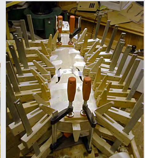
Right: Glowing of top with help of special clamps
